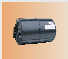
Consists of a centrifugal fan with double intake in nylon. The rotors are statically and dynamically balanced and are directly splined onto the motor shaft. Type monophase (230V, 50Hz) with condenser permanently installed and auto-transformer with 6 speeds 3 connected to the terminal board on the internal structure. The motor is installed on elastic antivibration supports and is built to comply with the IP21 safety rating.
