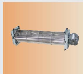
This unit is made of an aluminum, spiral, tangential impeller, equipped with antivibration, rubber bearing. The impeller is statically and dynamically balanced and is coupled with an engine, hold by a metallic bearing with antivibration devices.
